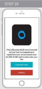
This will allow you to manually connect the Wi-Fi Bridge to your App. Press "Scan QR Code" You must allow The Automate Pulse app rights to use your smartphone/ tablet camera when prompted.
